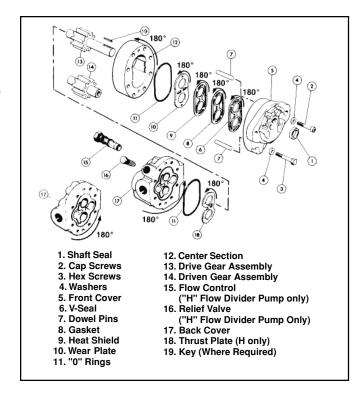
If the pump is an "H" series, install the thrust plate into the center section, orienting the side with the bar in line with the vent hole, ensuring that the bronze side faces the gears.
